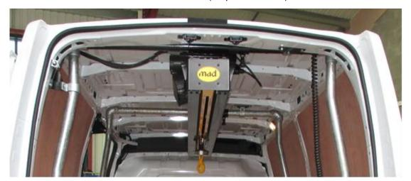
3.4.32 Now align the frame properly and check that, for all connector pieces, the marking on the tube is still just visible. If the marking is more than 2 mm from the edge of the connector piece, the tube has not been inserted sufficiently, and the frame is thus weakened.
