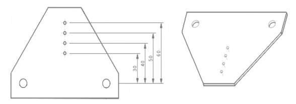
3.2.2 **130 triangular plate:** distance from the frame to the roof member varies from between 70 and 100 mm.
