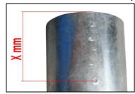
piece. A line or scratch must be put at "x" mm from the new cut. Where "x" is:
