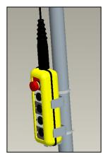
The handheld unit can be kept in the bracket for this purpose. The bracket should be installed on the post of the rear frame by using the two pipe clamps. The location can be freely selected by the end user. The connecting cable is sufficiently long to fasten the support for the handheld unit on both the left and the right post even when asymmetrically installing the EasyLoad.
